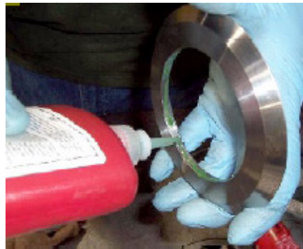
FIGURE 7-7 – LOCTITE 620 TO SLINGER
