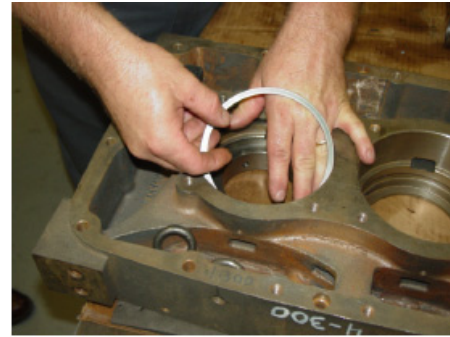
FIGURE 7-2 – INSTALL RETAINING RING
