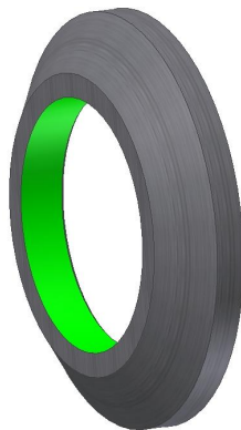
Figure 7-7 – LOCTITE 620 APPLIED TO INTERNAL SLINGER
